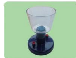
SM827 电解槽 Electrolytic tank
